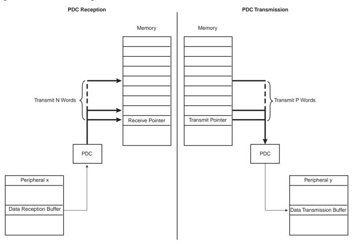
The PDC has data transfer ports which connect to the ASB and the AMBA Bridge. It is programmed via the APB. The ASB bus request and grant signals are used to request bus access, and to detect when that access has been granted according to the standard AMBA bus arbitration scheme.
