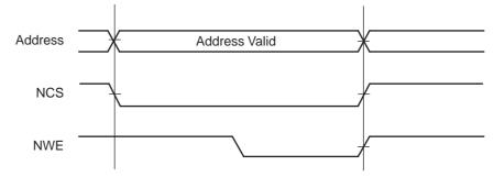
NWE (or NWR0, NWR1) goes high at the end of the write cycle, this is not true if a wait state is asserted.
