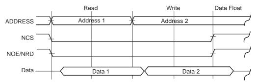
Figure 27. Sequential Early Read Access on the Same Chip Select with No Wait State
