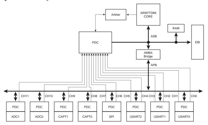
Each PDC channel, with a start address and a counter (number of words), can automatically put/get a block of transmitted words in/from a specific memory area. Each peripheral that transfers data can have a channel corresponding to a Peripheral Data Controller channel.
