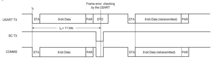
If a PDC transfer is used to send a data byte to the card, the PDC counter will not be decremented and the PDC memory pointer will not be incremented until the card has received a correct byte or the maximum repetition time has been reached.
