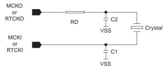
If the crystal recommended capacitor Cx is greater than 10 pF, then C1 and C2 must be added. Cx can be approximated to:  $Cx = \frac{C1 \times C2}{C1 + C2}$ .
