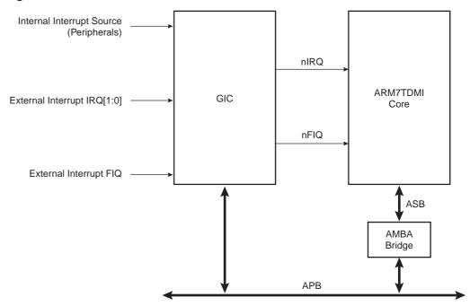
An 8-level priority encoder allows the user to define the priority between the different nIRQ interrupt sources. The internal interrupt sources are programmed to be level sensitive or edge triggered. The external interrupt sources can be programmed to be positive or negative edge triggered or high or low level sensitive.
