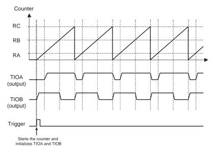
Generation of Two Identical Outof-phase Square-wave Signals TIOAx is toggled each time the counter reaches RA value, TIOBx each time the counter reaches RC value.
