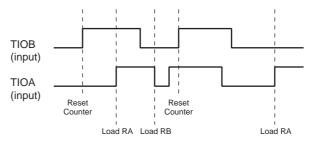
Measure Duration between Two Successive Rising TIOA Edges A TIOBx rising edge resets and starts the counter. The first rising TIOAx edge after the reset loads RA and a second loads RB. RA contains the phase between TIOBx and TIOAx. (RB-RA) is the period of the TIOAx pulse.
