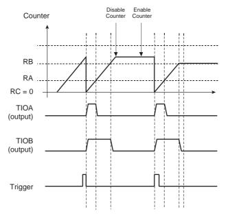
Trigger on TIOB Input Pin
