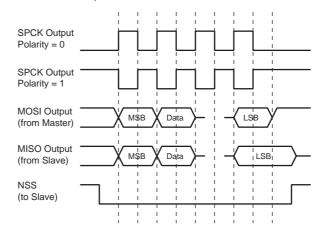
Figure 67. SPI in Master Mode, Phase = 1
