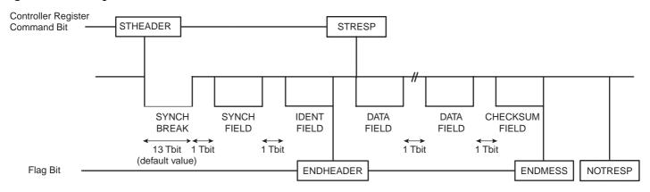
In Figure 56 above, unless the master has to file the "Response", no bits are to be set on the Control Register to wait for the slave's data field.
