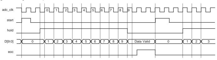
When start is high, the cell is reset and the internal clock is inhibited. The D[9:0] signal is at 512, so the internal ADC output is at (VREFP - GND)/2. The hold output is low, so the input voltage at the Sample and Hold stage of the comparator is sampled.
