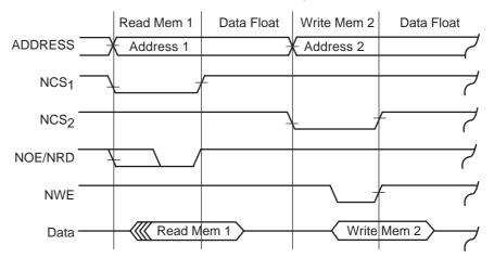
Figure 24. Read and Write Access on Different Chip Select with NTDF = 2
