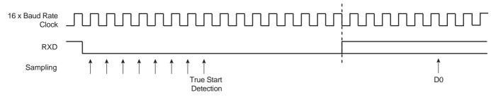
Figure 52. Asynchronous Mode Character Reception
