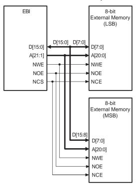
8-bit or 16-bit Access Device Connection
