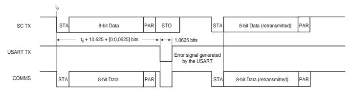
If a PDC transfer is used to receive a data byte from the card, the PDC counter will be decremented and the PDC memory pointer will be incremented even when a parity error is detected. The user must reconfigure the PDC memory pointer (decrement by 1) and counter (increment by 1) in order to receive all the remaining bytes.
