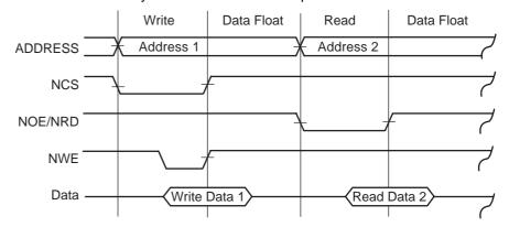
Figure 36. Write and Read on Different Chip Select
