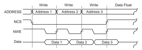
Figure 34. Sequential Write Access on Different Chip Select
