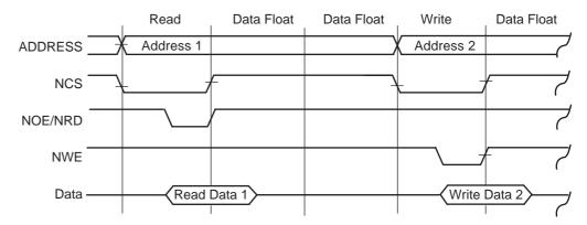
Figure 26. Sequential Early Read Access on the Same Chip Select with One Wait State
