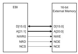
If users want to boot on a RAM memory for debug purposes, the RAM memory should be connected the same way as a flash memory (NUB and NLB of the RAM memory connected to the ground) to emulate a pure 16-bit Flash memory as shown in Figure 13.
