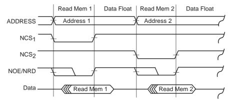
Figure 30. Sequential Standard Read Access on the Same Chip Select with One Wait State
