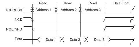
Figure 28. Sequential Read Access on Different Chip Select with NTDF = 2
