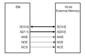
In the same configuration as shown in Figure 9 above, it is possible to connect 2x8-bit memory devices with 16-bit access. The configuration shown in Figure 10 on page 28 demonstrates how to interface the EBI with 2x8-bit memories (for example 2x8-bit ROM memory) as a 16-bit memory page.
