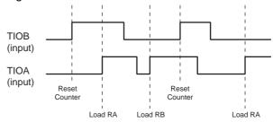
Measure the Duration of a TIOA Pulse or Period (TIOB Not Used) A TIOAx falling edge resets, starts the counter and loads RB if RA is already loaded. A TIOAx rising edge loads RA. RA contains the duration of a TIOAx pulse (low level). RB contains the duration of the TIOAx period.
