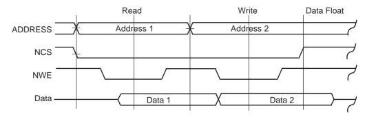
Figure 33. Sequential Write Access on the Same Chip Select with No Wait State
