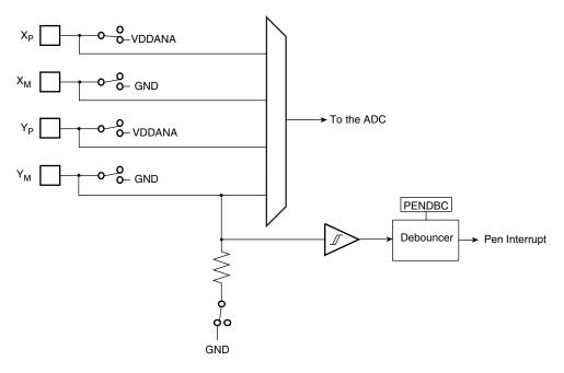
The Touch Screen Pen Detect can be used to generate a TSADCC interrupt to wake up the system or it can be programmed to trig a conversion, so that a position can be measured as soon as a contact is detected if the TSADCC is programmed for an operating mode involving the Touch Screen.
