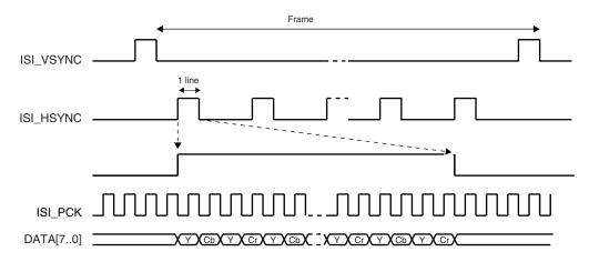
Figure 38-4. SAV and EAV Sequence Synchronization
