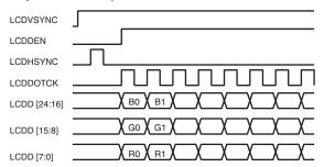
Figure 44-7. Single Scan Monochrome and Color 4-bit Panel Timing (First Line Expanded View)
