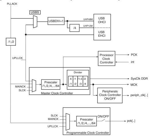
Figure 25-1. AT91SAM9G45 Power Management Controller Block Diagram
