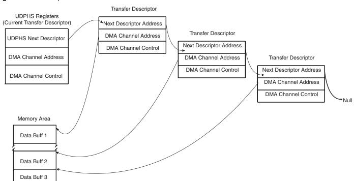
**Figure 37-6.** Example of DMA Chained List:
