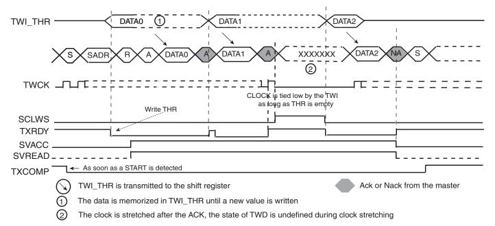
Notes: 1. TXRDY is reset when data has been written in the TWI\_THR to the shift register and set when this data has been acknowledged or non acknowledged.
