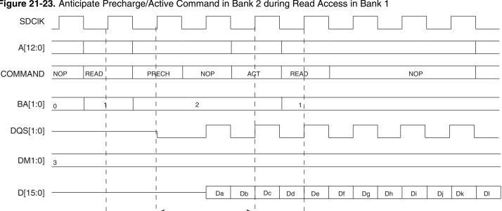
Figure 21-23. Anticipate Precharge/Active Command in Bank 2 during Read Access in Bank 1
