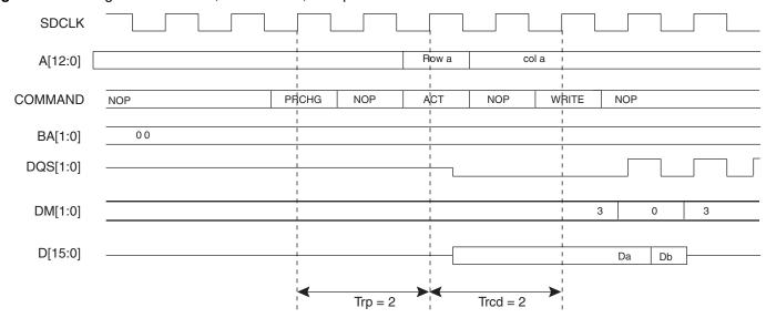
Figure 21-3. Single Write Access, Row Closed, DDR2-SDRAM Device
