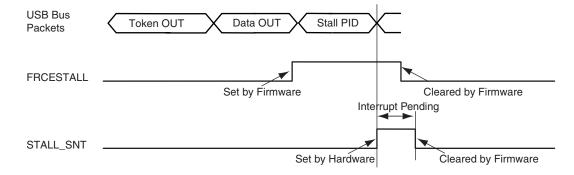
Figure 37-17. Stall Handshake Data IN Transfer
