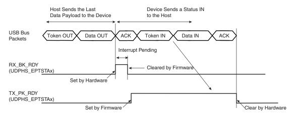
**Note**: Before proceeding to the status stage, the software should determine that there is no risk of extra data from the host (data stage). If not certain (non-predictable data stage length), then the software should wait for a NAK-IN interrupt before proceeding to the status stage. This precaution should be taken to avoid collision in the FIFO.
