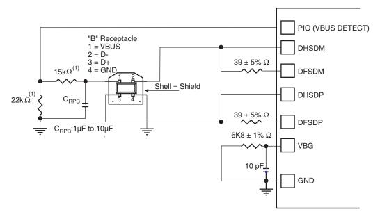
Notes: 1. The values shown on the  $22k\Omega$  and  $15k\Omega$  resistors are only valid with 3V3 supplied PIOs.
