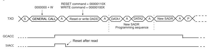
This method allows the user to create an own programming sequence by choosing the programming bytes and the number of them. The programming sequence has to be provided to the master.
