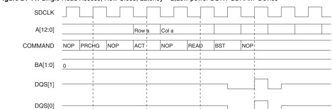
Figure 21-11. Single Read Access, Row Close, Latency = 2, Low-power DDR1-SDRAM Device
