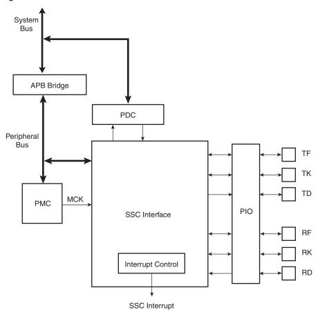
Figure 32-2. Block Diagram
