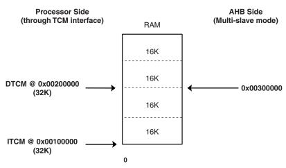
Within the 64 Kbyte SRAM size available, the amount of memory assigned to each block is software programmable according to Table 6-1.
