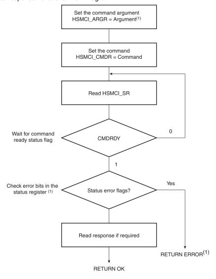
Figure 34-7. Command/Response Functional Flow Diagram
