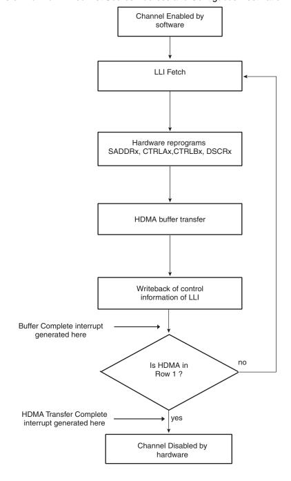
Figure 40-16. DMAC Transfer Flow for Linked List Source Address and Contiguous Destination Address
