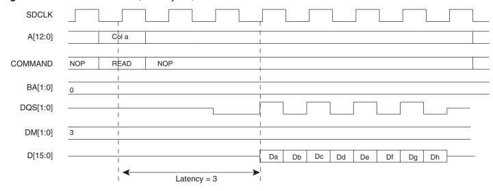
Figure 21-16. Burst Read Access, Latency = 2, SDR-SDRAM Devices
