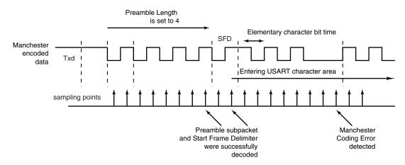
When the start frame delimiter is a sync pattern (ONEBIT field at 0), both command and data delimiter are supported. If a valid sync is detected, the received character is written as RXCHR
