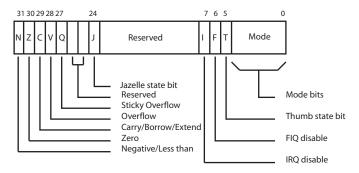
Figure 9-2 shows the status register format, where:
