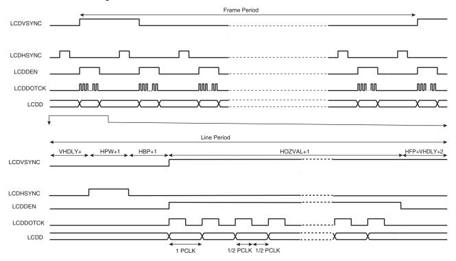
Figure 44-4. TFT Panel Timing, CLKMOD = 0, VPW = 2, VBP = 2, VFP = 1
