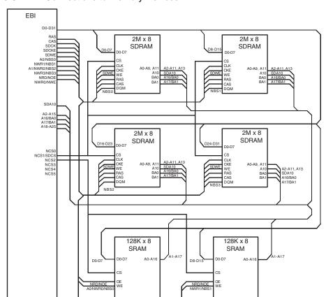
Figure 19-3. EBI Connections to Memory Devices
