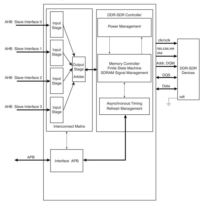
DDRSDRC is partitioned in two blocks (see Figure 21-1):
