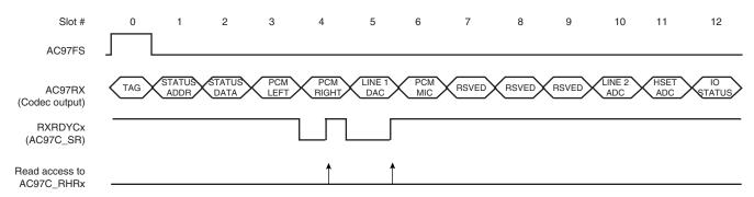
If the previously received data has not been read by the application, the new data overwrites the data already waiting in AC97C\_CxRHR, therefore the OVRUN flag in AC97C\_CxSR is raised. The application can either poll the OVRUN flag in AC97C\_CxSR or wait for an interrupt notice. The interrupt remains active until the OVRUN flag in AC97C\_CxSR is set.
