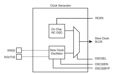
RCEN, OSC32EN, OSCSEL and OSC32BYP bits are located in the Slow Clock Control Register (SCKCR) located at address 0xFFFFD50 in the backed up part of the System Controller and so are preserved while VDDBU is present.
