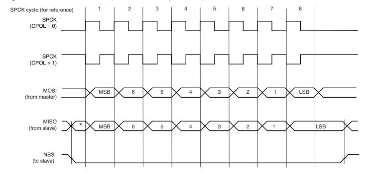
Figure 29-5. SPI Transfer Format (NCPHA = 0, 8 bits per transfer)
