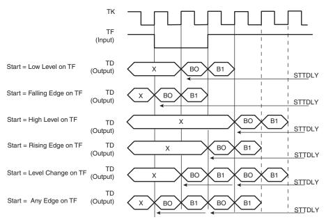
Figure 32-12. Receive Pulse/Edge Start Modes
