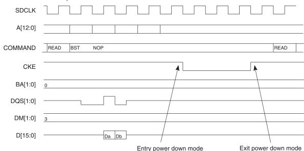
Figure 21-20. Power-down Entry/Exit, Timeout = 0
