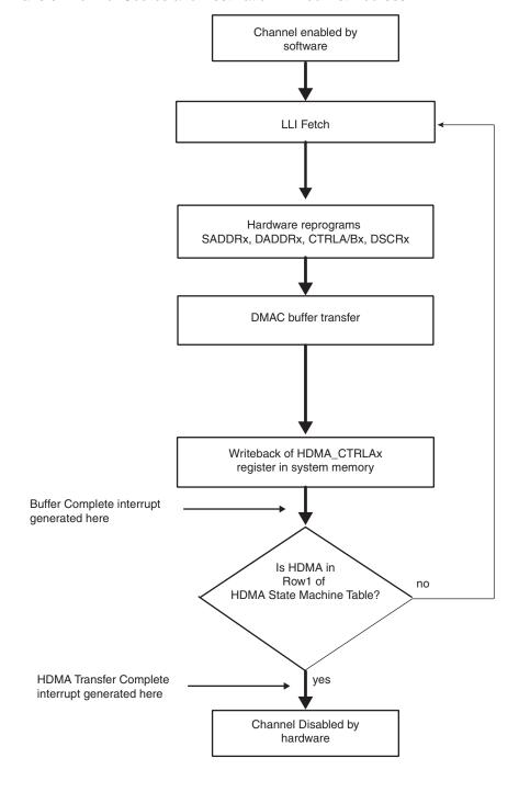
Figure 40-8. DMAC Transfer Flow for Source and Destination Linked List Address
