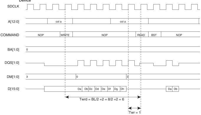
In the case of a single write access, write operation should be interrupted by a read access but DM must be input 1 cycle prior to the read command to avoid writing invalid data. See Figure 21-9 on page 236.
