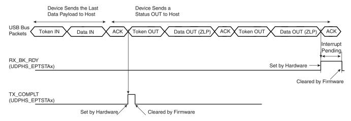
Note: A NAK handshake is always generated at the first status stage token.
