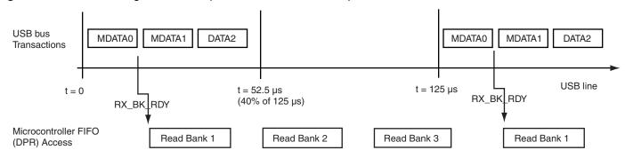
USB 2.0 supports individual High Speed isochronous endpoints that require data rates up to 192 Mb/s (24 MB/s): 3x1024 data bytes per microframe.
