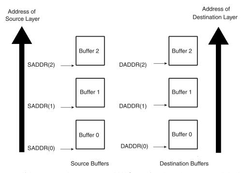
If the user needs to execute a DMAC transfer where the source and destination address are contiguous but the amount of data to be transferred is greater than the maximum buffer size DMAC\_CTRLAx.BTSIZE, then this can be achieved using the type of multi-buffer transfer as shown in Figure 40-7 on page 926.
