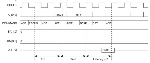
Figure 21-14. Burst Read Access, Latency = 2, Low-power DDR1-SDRAM Devices
