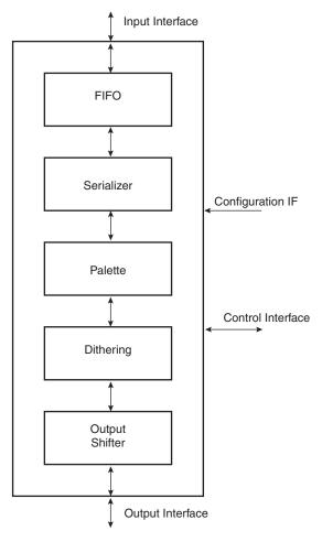
This module transforms the data read from the memory into a format according to the LCD module used. It has four different interfaces: the input interface, the output interface, the configuration interface and the control interface.
