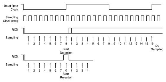
Figure 31-13. Asynchronous Character Reception
