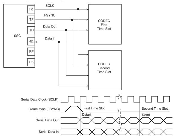
Figure 32-21. Time Slot Application Block Diagram
