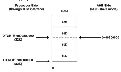
Within the 64 Kbyte SRAM size available, the amount of memory assigned to each block is software programmable according to Table 7-1.
