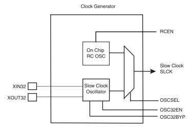
After a VDDBU power on reset, the default configuration is RCEN = 1, OSC32EN = 0 and OSC-SEL = 0 allowing the system to start on the internal RC oscillator.
