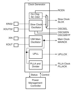
Figure 8-2. Clock Generator Block Diagram
