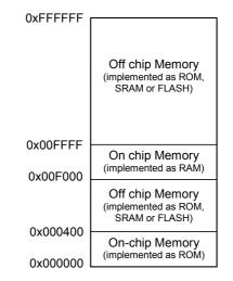
The figure below shows a typical Program Memories connections in system with DP80390 Microcontroller core.
