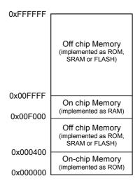
The figure below shows a typical Program Memories connections in system with DP80390CPU Microcontroller core.
