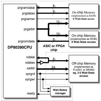
The described above implementation should be treated as an example. All Program Memory spaces are fully configurable. For timing-critical applications whole program code can be implemented as on-chip ROM and (or) RAM and executed without Wait-States, but for some other applications whole program code can be implemented as off-chip ROM or FLASH and executed with required number Wait-State cycles.
