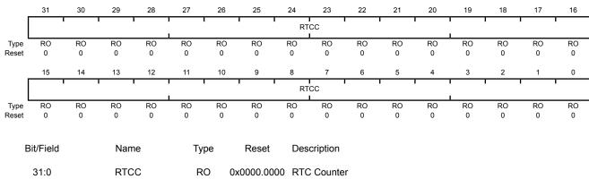
A read returns the 32-bit counter value. This register is read-only. To change the value, use the HIBRTCLD register.
