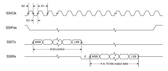
Figure 26-15. SSI Timing for SPI Frame Format (FRF=00), with SPH=1
