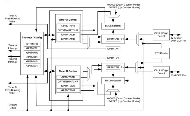
**Note:** In Figure 11-1 on page 368, the specific Capture Compare PWM (CCP) pins available depend on the Stellaris<sup>®</sup> device. See Table 11-1 on page 368 for the available CCP pins and their timer assignments
