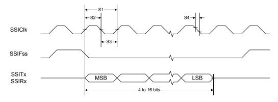
Figure 26-14. SSI Timing for MICROWIRE Frame Format (FRF=10), Single Transfer
