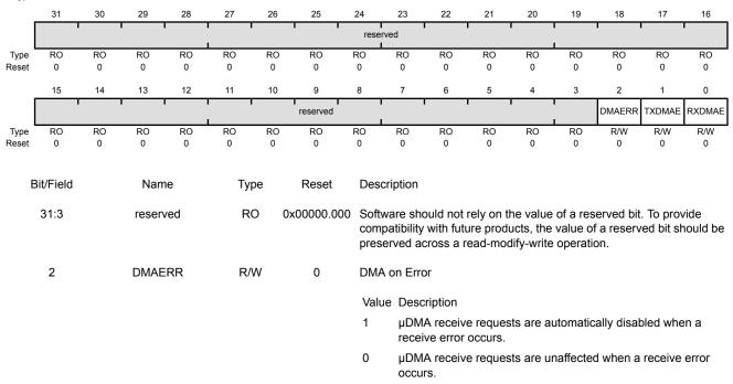
TXDMAE R/W 0 Transmit DMA Enable
