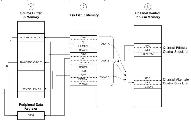
Figure 9-5. Peripheral Scatter-Gather, Setup and Configuration
