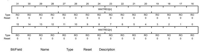
These bits provide the channel wait-on-request status. Bit 0 corresponds to channel 0.
