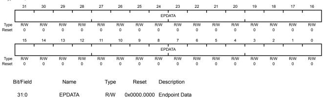
Writing to this register loads the data into the Transmit FIFO and reading unloads data from the Receive FIFO.
