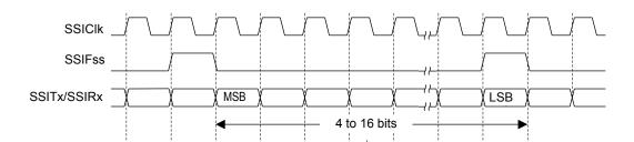
Figure 15-3. TI Synchronous Serial Frame Format (Continuous Transfer)
