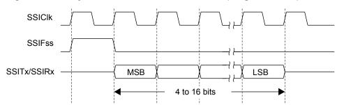
Figure 15-2. TI Synchronous Serial Frame Format (Single Transfer)
