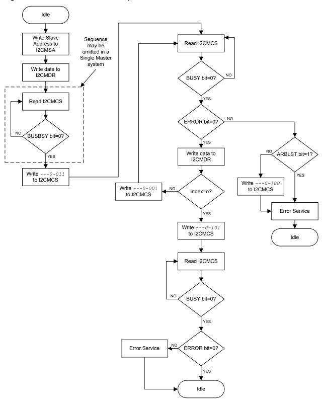
Figure 16-9. Master TRANSMIT with Repeated START
