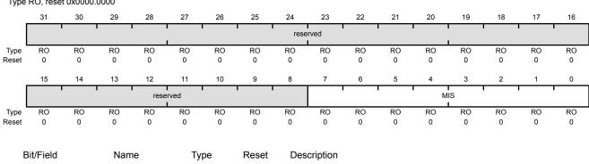
31.8 reserved RO 0x0000.00 Software should not rely on the value of a reserved bit. To provide compatibility with future products, the value of a reserved bit should be preserved across a read-modify-write operation.
