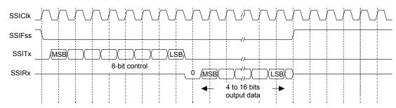
Figure 15-10. MICROWIRE Frame Format (Single Frame)
