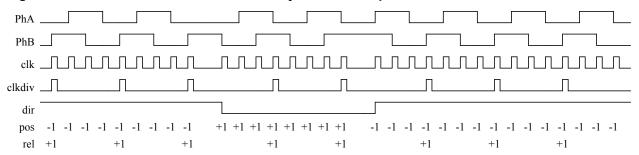
The period of the timer is configurable by specifying the load value for the timer in the **QEI Timer Load (QEILOAD)** register. When the timer reaches zero, an interrupt can be triggered, and the hardware reloads the timer with the **QEILOAD** value and continues to count down. At lower encoder speeds, a longer timer period is required to be able to capture enough edges to have a meaningful result. At higher encoder speeds, both a shorter timer period and/or the velocity predivider can be used.
