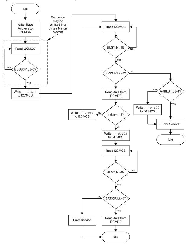
Figure 16-10. Master RECEIVE with Repeated START
