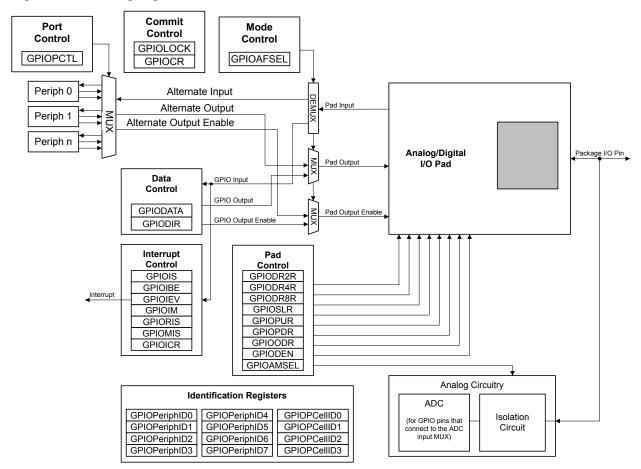
Figure 10-2. Analog/Digital I/O Pads
