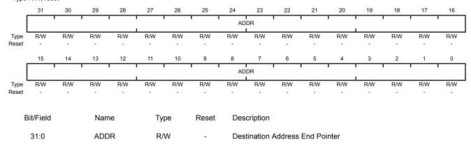
This field points to the last address of the  $\mu DMA$  transfer destination (inclusive). If the destination address is not incrementing (the DSTINC field in the **DMACHCTL** register is 0x3), then this field points at the destination location itself (such as a peripheral data register).
