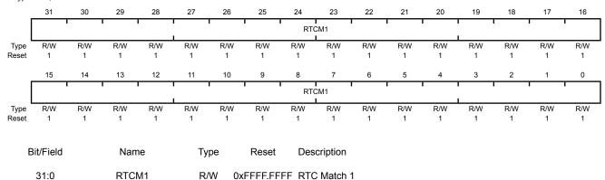
A write loads the value into the RTC match register.
