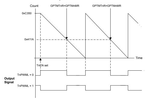
Figure 11-4. 16-Bit PWM Mode Example
