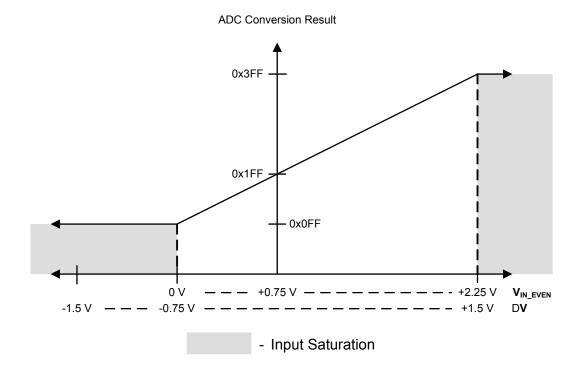
Figure 13-7. Differential Sampling Range,  $V_{IN\_ODD}$  = 2.25 V
