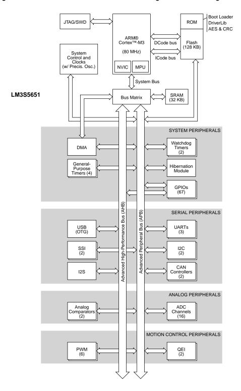
Figure 1-1. Stellaris<sup>®</sup> LM3S5651 Microcontroller High-Level Block Diagram
