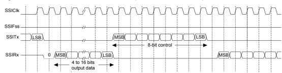
Figure 15-11. MICROWIRE Frame Format (Continuous Transfer)
