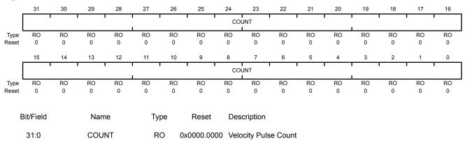
The running total of encoder pulses during this velocity timer period.
