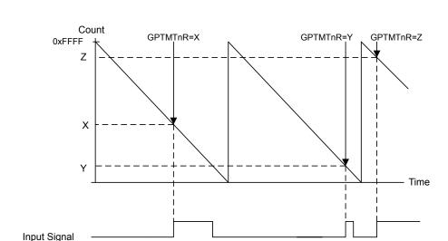
Figure 11-3. 16-Bit Input Edge-Time Mode Example
