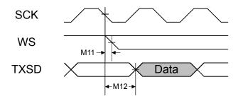
Figure 26-18. I<sup>2</sup>S Master Mode Receive Timing
