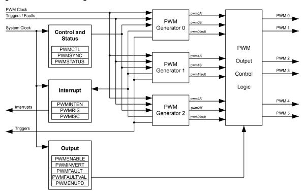
Figure 21-1. PWM Unit Diagram
