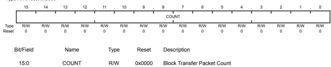
Sets the number of packets of the size defined by the  ${\tt MAXLOAD}$  bit field that are to be transferred in a block transfer.
