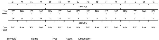
31:0 CHALT[n] R/W Channel [n] Alternate Assignment Select
