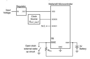
Figure 7-3. Clock Source Using Dedicated Oscillator and VDD3ON Mode
