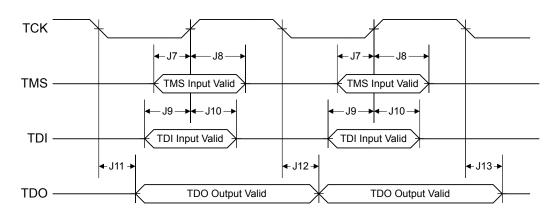
Figure 26-3. JTAG Test Access Port (TAP) Timing
