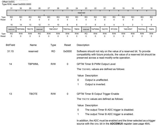
Software should not rely on the value of a reserved bit. To provide compatibility with future products, the value of a reserved bit should be
