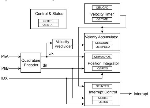
Figure 22-1. QEI Block Diagram
