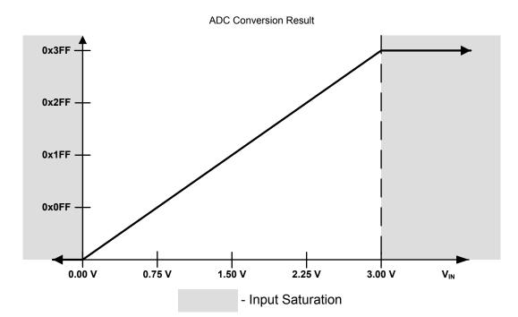
Figure 13-3. Internal Voltage Conversion Result
