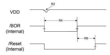
Figure 26-7. Software Reset Timing
