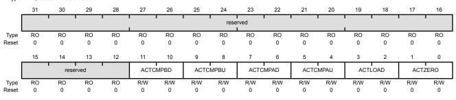
Bit/Field Description Type Reset 31:12 reserved RO 0.0000x0 Software should not rely on the value of a reserved bit. To provide compatibility with future products, the value of a reserved bit should be preserved across a read-modify-write operation.
