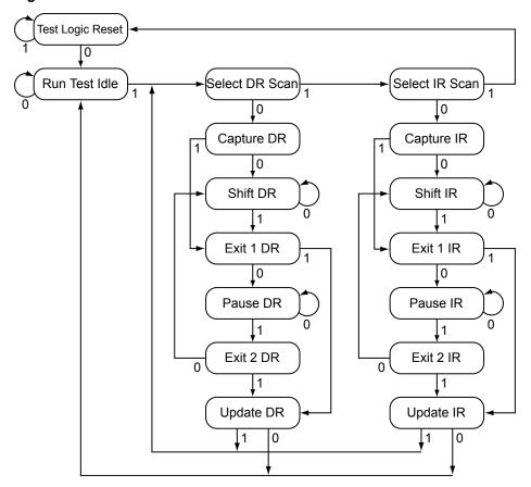
Figure 5-2. Test Access Port State Machine
