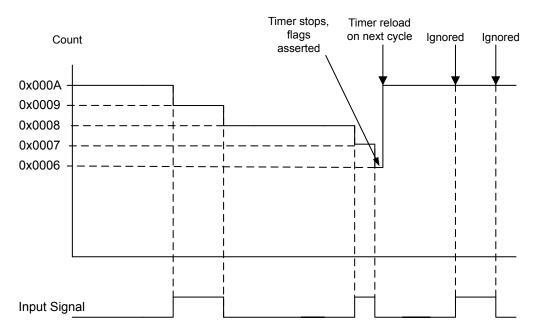
Figure 11-2. 16-Bit Input Edge-Count Mode Example
