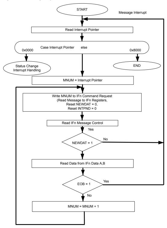
Figure 18-3. Message Objects in a FIFO Buffer
