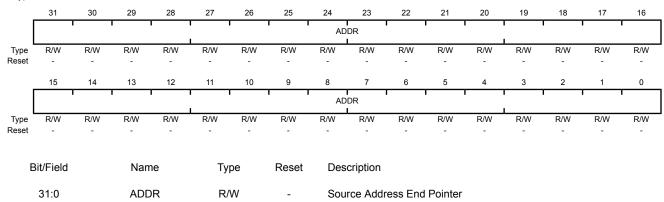
This field points to the last address of the  $\mu DMA$  transfer source (inclusive). If the source address is not incrementing (the SRCINC field in the **DMACHCTL** register is 0x3), then this field points at the source location itself (such as a peripheral data register).
