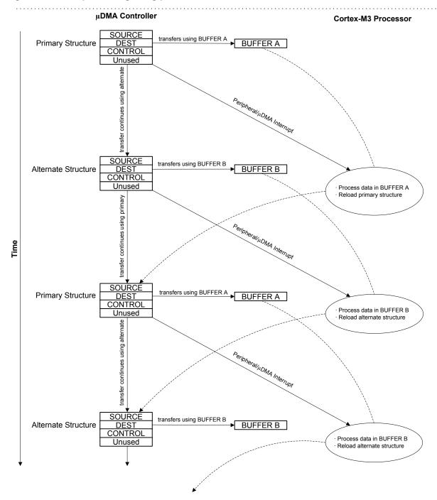
Figure 9-2. Example of Ping-Pong µDMA Transaction
