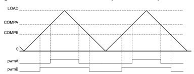
Figure 21-5. PWM Generation Example In Count-Up/Down Mode
