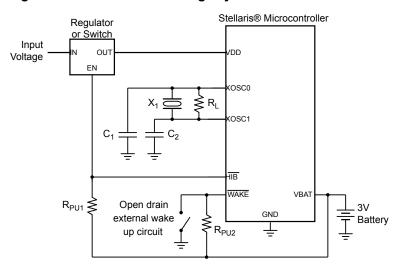
Figure 7-2. Clock Source Using Crystal
