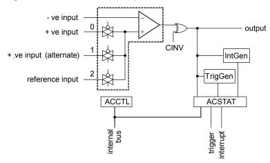
A comparator is configured through two status/control registers, Analog Comparator Control (ACCTL) and Analog Comparator Status (ACSTAT). The internal reference is configured through one control register, Analog Comparator Reference Voltage Control (ACREFCTL). Interrupt status and control are configured through three registers, Analog Comparator Masked Interrupt Status (ACMIS), Analog Comparator Raw Interrupt Status (ACRIS), and Analog Comparator Interrupt Enable (ACINTEN).
