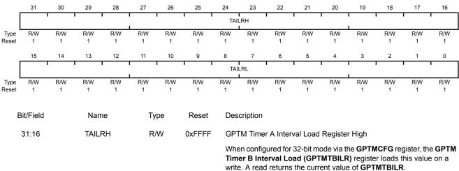
In 16-bit mode, this field reads as 0 and does not have an effect on the state of GPTMTBILR.
