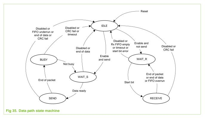
• IDLE: The data path is inactive, and the MD3:0 outputs are in hi-Z. When the data control register is written and the enable bit is set, the DPSM loads the data counter with a new value and, depending on the data direction bit, moves to either the WAIT\_S or WAIT\_R state.
