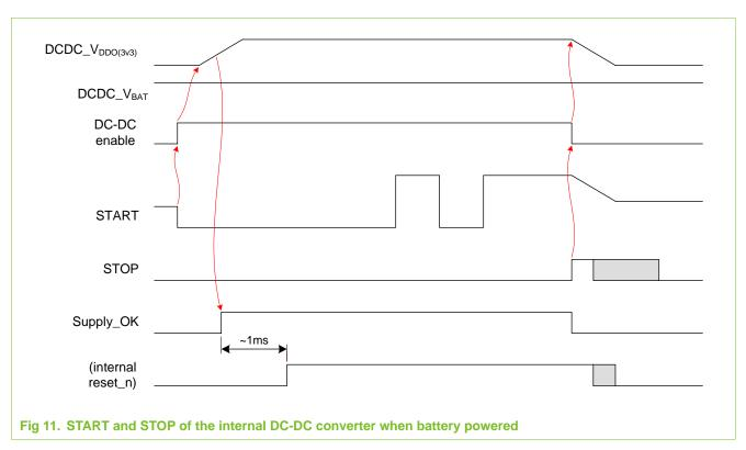
A positive edge on the STOP signal causes the DC-DC converter to shut off and the internal reset to be asserted.
