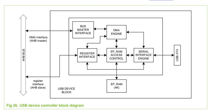
The architecture of the USB device controller is shown in Figure 19–26.
