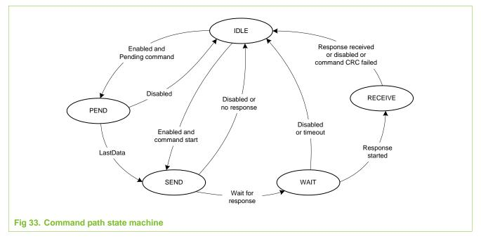
When the WAIT state is entered, the command timer starts running. If the timeout is reached before the CPSM moves to the RECEIVE state, the timeout flag is set and the IDLE state is entered.
