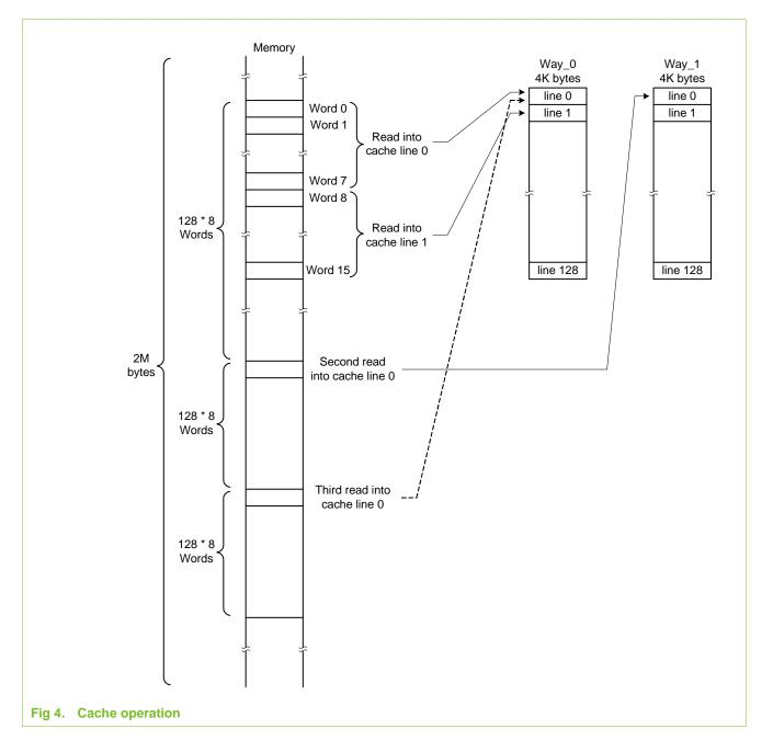
The cache has 16 configurable pages, each being 2 megabytes in size. The cache treats these 16 pages as if they occupy the bottom 32 Megabytes of the system memory map, which is their default mapping. The cache can re-map any of these pages such that the physical address is above the lower 32 megabytes.
