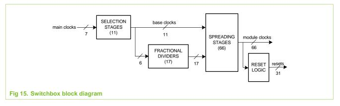
The selection stages select among the main clocks, although they are more complex than simple selectors in order to avoid glitches when they are being dynamically switched between main clocks. The outputs of the selection stages are called "base clocks". Some selection stages and base clocks are dedicated to a particular spreading stage and
