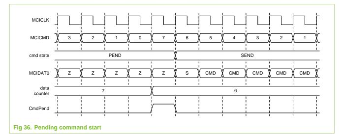
The data block counter determines the end of a data block. If the counter is zero, the end-of-data condition is TRUE (see <u>Section 24–5.10 on page 280</u> for more information).
