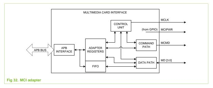
The MCI adapter is a multimedia/secure digital memory card bus master that provides an interface to a multimedia card stack or to a secure digital memory card. It consists of five subunits:
