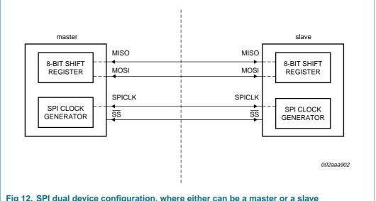
Fig 12. SPI dual device configuration, where either can be a master or a slave
