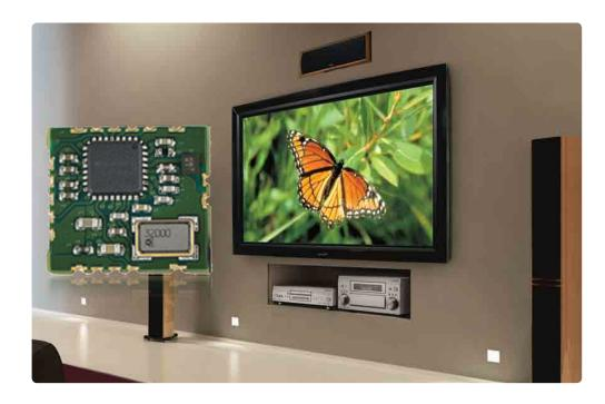
The ZM4102 represents the fourth-generation of Z-Wave® wireless technology, and is ideal for easily adding Z-Wave® control and status capabilities to home control, home security monitoring, and home energy management products. The ZM4102 module includes a Z-Wave® chip and external components required to implement a complete, drop-in solution.
