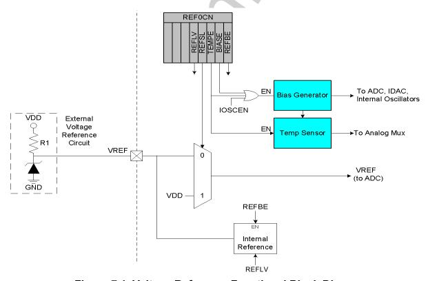
Figure 7.1. Voltage Reference Functional Block Diagram
