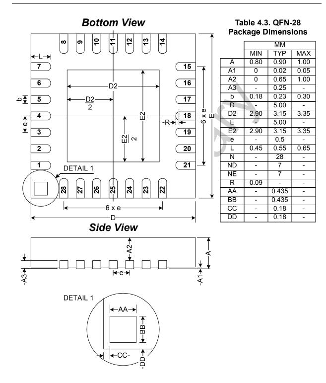
Figure 4.4. QFN-28 Package Drawing
