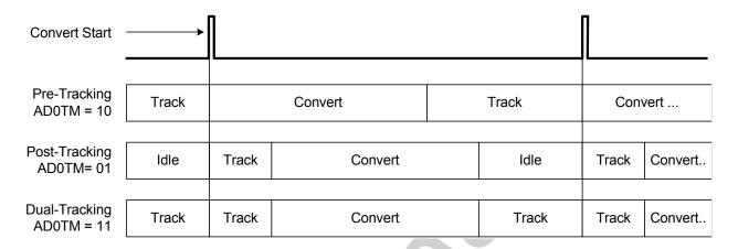
Figure 5.3. ADC0 Tracking Modes
