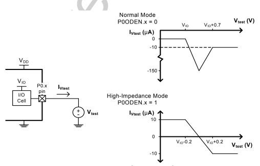
Figure 18.5. Port 0 Input Overdrive Current Range
