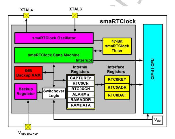
Figure 1.10. smaRTClock Block Diagram
