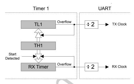
Figure 22.2. UARTO Baud Rate Logic
