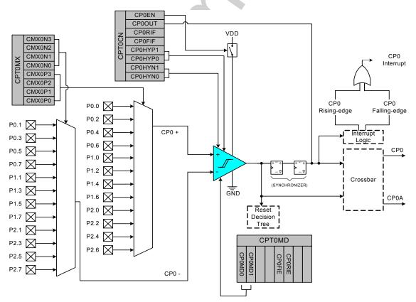
Figure 9.1. Comparator Functional Block Diagram
