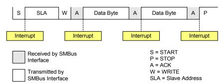
Figure 21.5. Typical Master Transmitter Sequence
