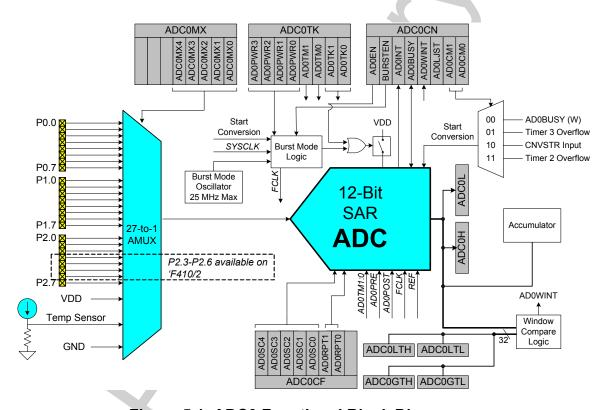
Figure 5.1. ADC0 Functional Block Diagram
