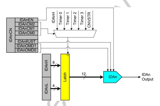
Figure 6.1. IDAC Functional Block Diagram
