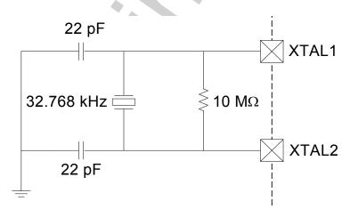
Figure 19.2. 32.768 kHz External Crystal Example
