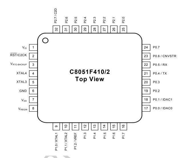
Figure 4.1. LQFP-32 Pinout Diagram (Top View)
