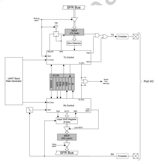
Figure 22.1. UART0 Block Diagram
