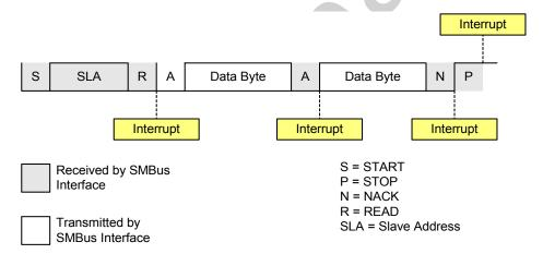
Figure 21.8. Typical Slave Transmitter Sequence
