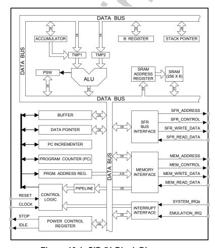
Figure 10.1. CIP-51 Block Diagram
