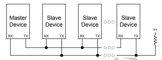
Figure 22.6. UART Multi-Processor Mode Interconnect Diagram
