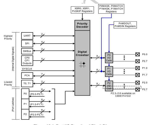
Figure 18.1. Port I/O Functional Block Diagram
