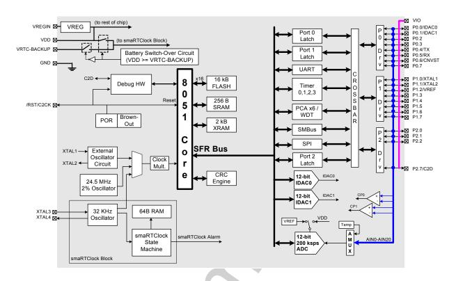
Figure 1.4. C8051F413 Block Diagram
