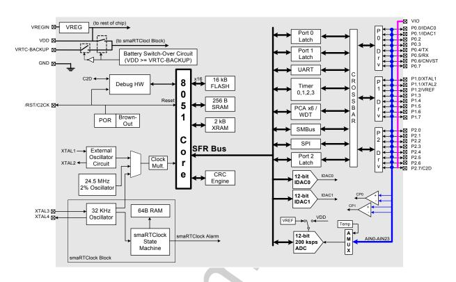
Figure 1.3. C8051F412 Block Diagram
