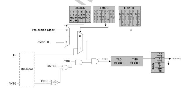
Figure 24.1. T0 Mode 0 Block Diagram
