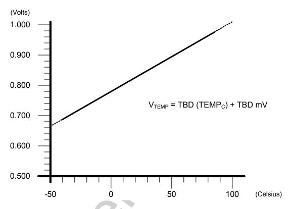
Figure 5.2. Typical Temperature Sensor Transfer Function
