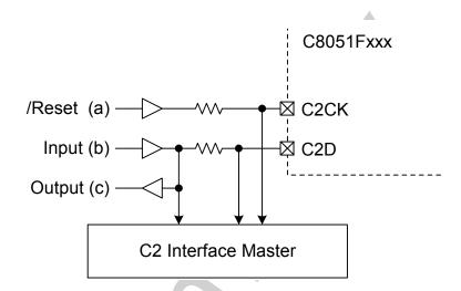
Figure 26.1. Typical C2 Pin Sharing
