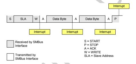
Figure 21.7. Typical Slave Receiver Sequence
