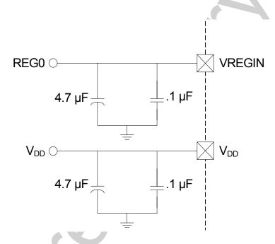
Figure 8.1. External Capacitors for Voltage Regulator Input/Output
