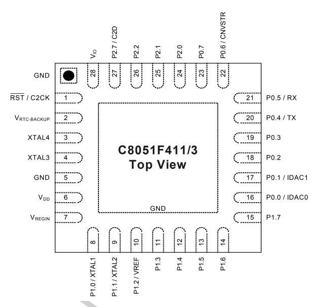
Figure 4.2. QFN-28 Pinout Diagram (Top View)
