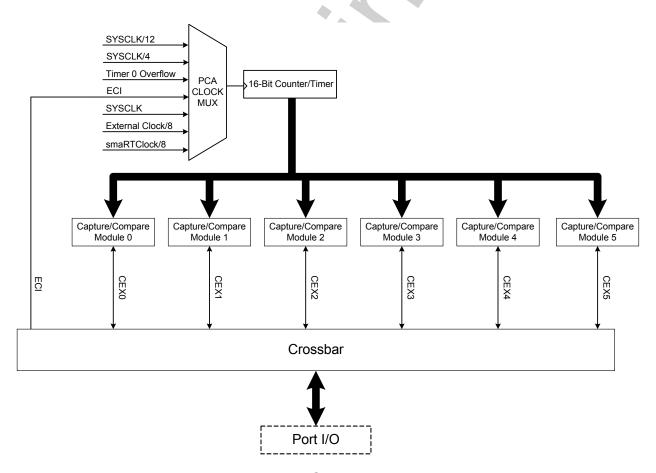
Figure 25.1. PCA Block Diagram
