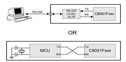
Figure 22.3. UART Interconnect Diagram
