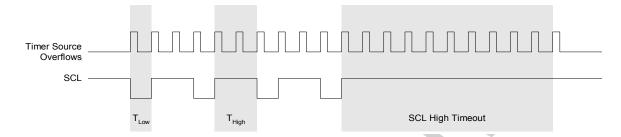
Figure 21.4. Typical SMBus SCL Generation
