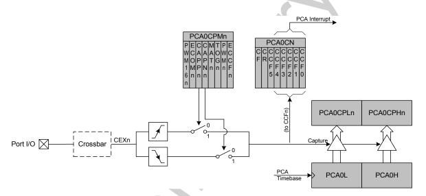
Figure 25.4. PCA Capture Mode Diagram
