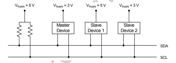
Figure 21.2. Typical SMBus Configuration
