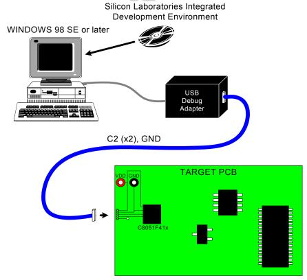
Figure 1.5. Development/In-System Debug Diagram
