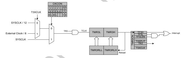
Figure 24.7. Timer 3 16-Bit Mode Block Diagram
