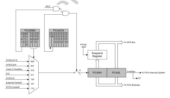
Figure 25.2. PCA Counter/Timer Block Diagram
