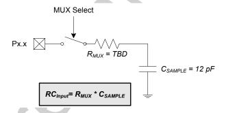
Figure 5.6. ADC0 Equivalent Input Circuits
