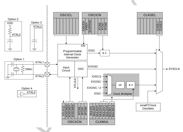
Figure 19.1. Oscillator Diagram
