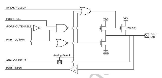
Figure 18.2. Port I/O Cell Block Diagram
