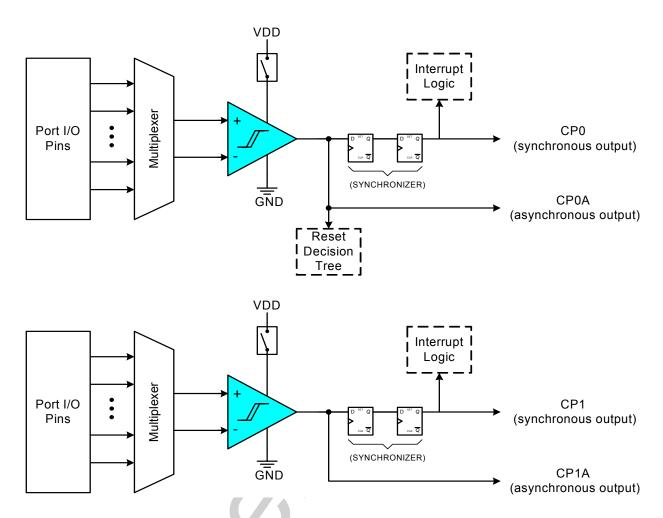
Figure 1.9. Comparators Block Diagram
