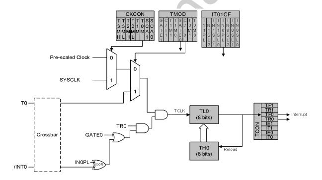
Figure 24.2. T0 Mode 2 Block Diagram
