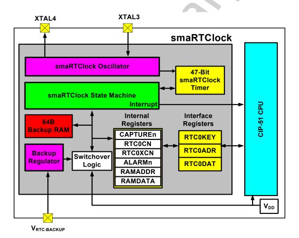
Figure 20.1. smaRTClock Block Diagram
