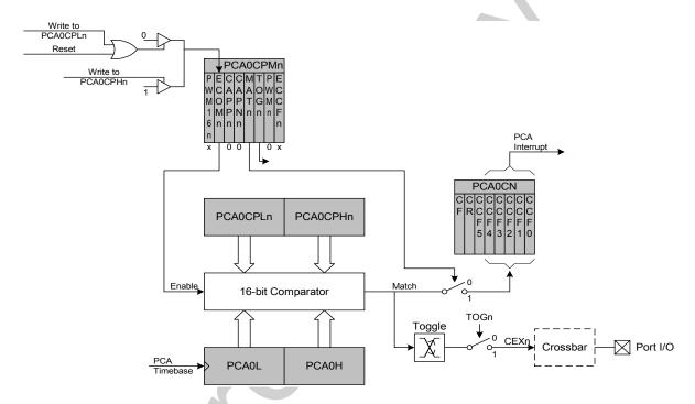
Figure 25.6. PCA High-Speed Output Mode Diagram
