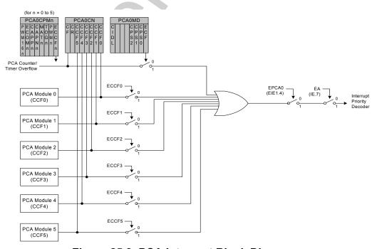
Figure 25.3. PCA Interrupt Block Diagram
