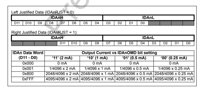
Figure 6.2. IDAC Data Word Mapping
