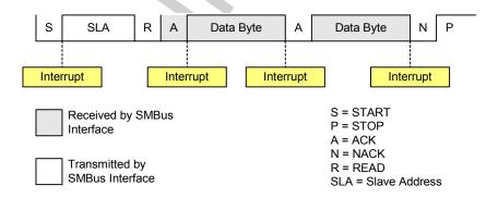
Figure 21.6. Typical Master Receiver Sequence
