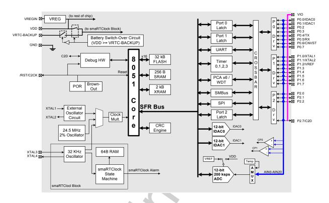
Figure 1.2. C8051F411 Block Diagram
