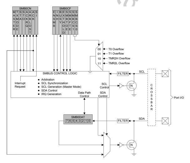
Figure 21.1. SMBus Block Diagram
