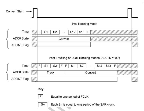
Figure 5.4. 12-Bit ADC Tracking Mode Example
