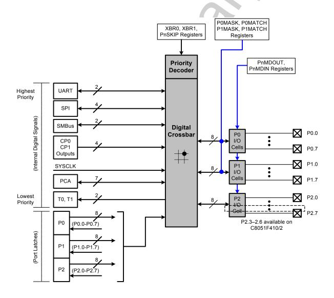
Figure 1.11. Port I/O Functional Block Diagram
