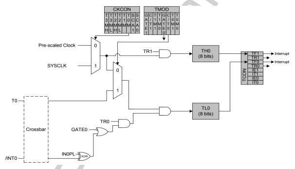
Figure 24.3. T0 Mode 3 Block Diagram
