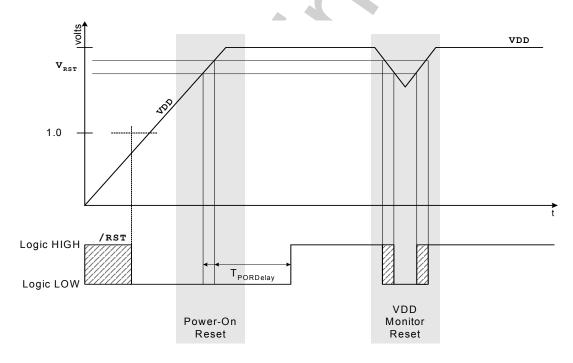
Figure 15.2. Power-On and V<sub>DD</sub> Monitor Reset Timing
