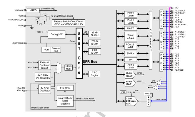
Figure 1.1. C8051F410 Block Diagram
