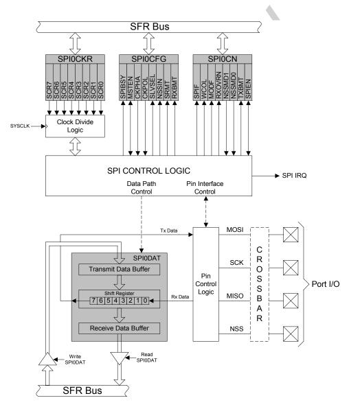
Figure 23.1. SPI Block Diagram
