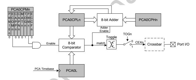
Figure 25.7. PCA Frequency Output Mode
