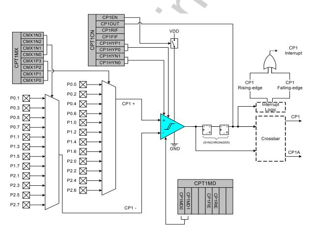
Figure 9.2. Comparator1 Functional Block Diagram
