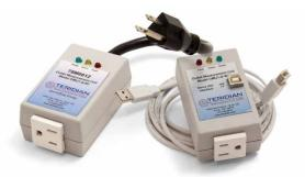
Teridian's Outlet Measurement Unit (OMU) is a compact demonstration kit employing the 78M6612 SOC. The 78M6612 monitors the AC line voltages, frequency, and load current. The embedded firmware calculates items such as RMS line voltage and RMS load current, watts, VA, VAR and power factor. The real time data is transmitted via the serial interface to a PC for display in a Windows<sup>®</sup> based Graphical User Interface.
