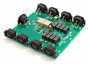
The 78M6618 evaluation board is a design example of a switched 8-outlet power distribution unit with per outlet metering. The board includes one 78M6618 IC, an AC-DC power supply, one AC input, eight switched outputs (relays), and connectors to the serial interfaces and DIO pins.
