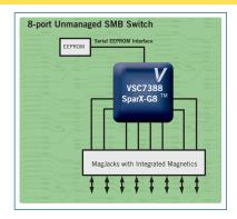
With its unique low power dissipation the VSC7388 enables fan less operation and thereby provides for higher system reliability and lower noise, both to the benefit of the user.
