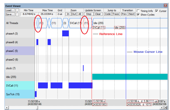
The Event Viewer displays thread, interrupt, and exception execution over time.
