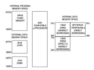
At power-up/reset code is executed from the 64Kx8 Flash memory mapped into the processor's internal ROM space. An extra 2Kx8 of Secondary Flash memory is mapped into the external data memory space.
