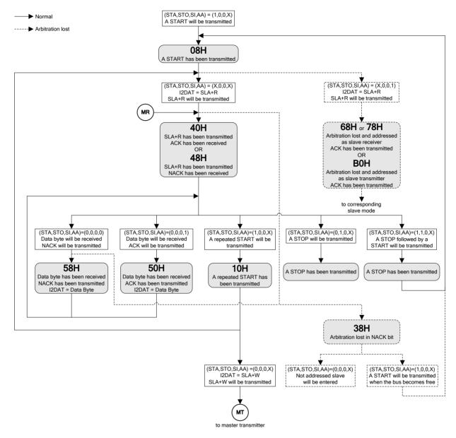
Figure 15.8. Flow and Status of Master Receiver Mode
