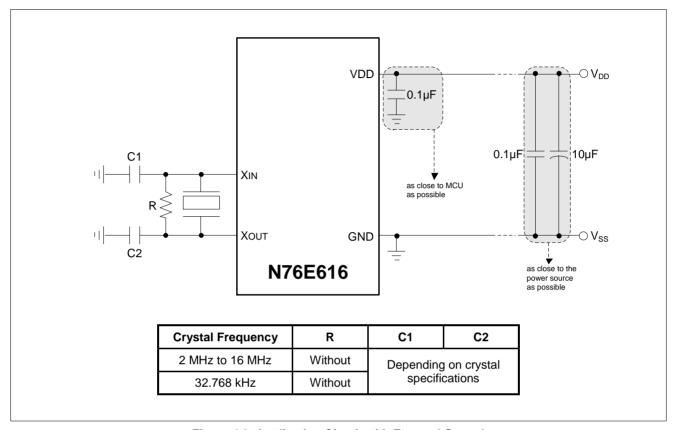
Figure 4.3. Application Circuit with External Crystal
