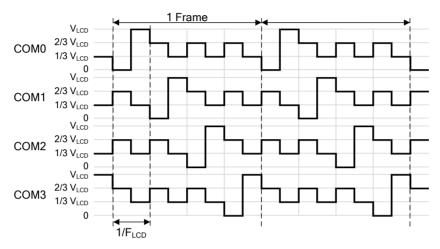
Figure 18.1. COM Driving Signals (1/4 Duty and 1/3 Bias)
