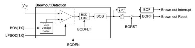
Figure 24.1. Brown-out Detection Block Diagram
