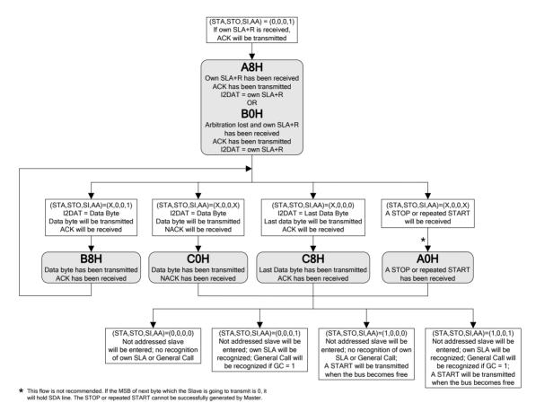
Figure 15.10. Flow and Status of Slave Transmitter Mode
