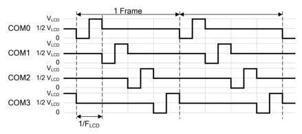
Figure 18.4. COM Driving Signals (1/4 Duty and 1/2 Bias)
