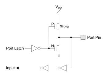
Figure 8.2. Push-Pull Mode Structure
