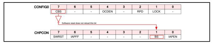
Figure 29.1. CONFIG0 Any Reset Reloading
