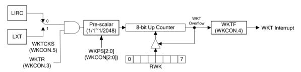
Figure 13.1. Self Wake-Up Timer Block Diagram
