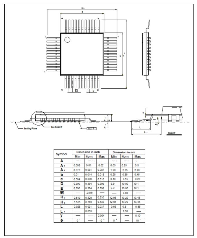
Figure 32.2 PQFP44 (10x10x2.0mm, footprint 3.2mm) Package Dimension
