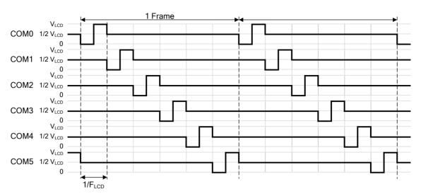
Figure 18.6. COM Driving Signals (1/6 Duty and 1/2 Bias)
