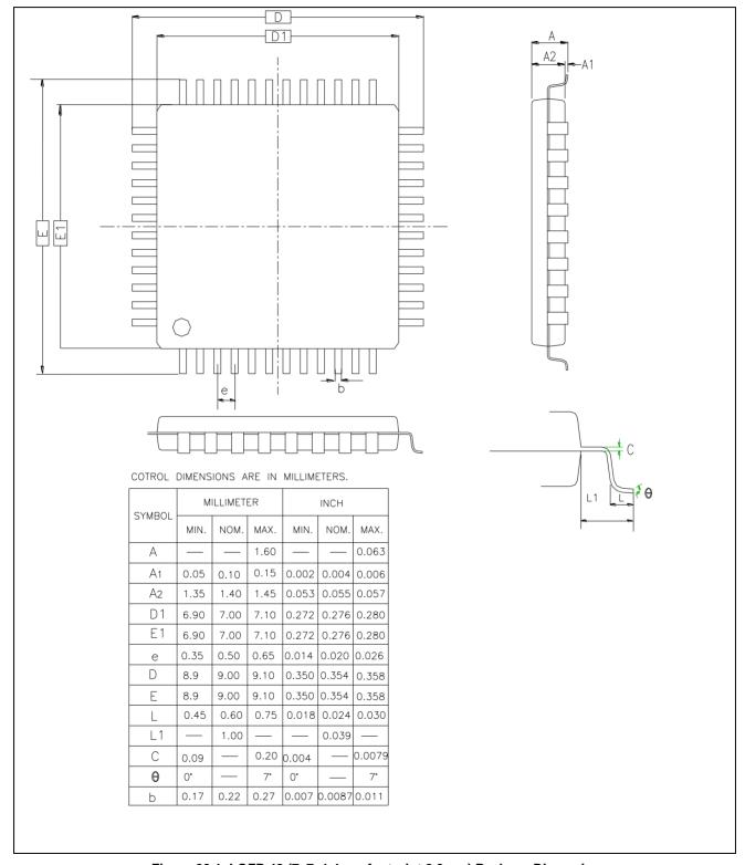
Figure 32.1. LQFP-48 (7x7x1.4mm footprint 2.0mm) Package Dimension
