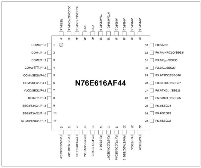
Figure 4.2 Pin Assignment of PQFP-44 Package
