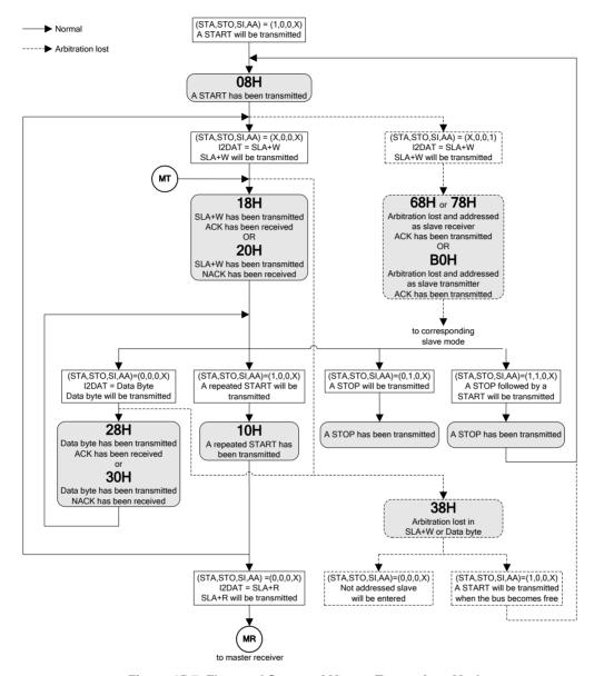
Figure 15.7. Flow and Status of Master Transmitter Mode
