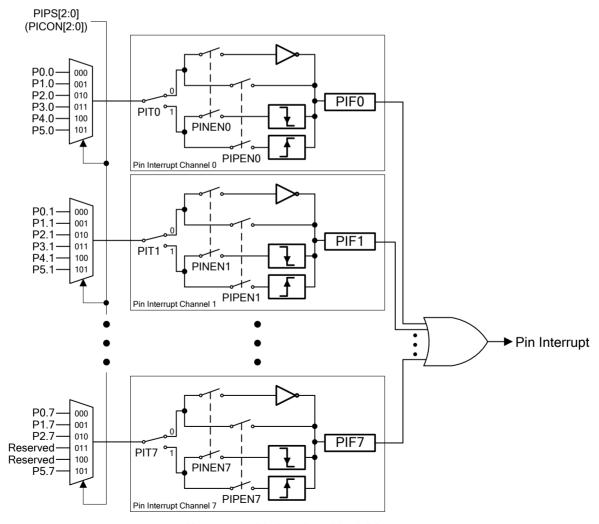
Figure 16.1. Pin Interface Block Diagram
