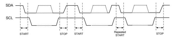
Figure 15.3. START, Repeated START, and STOP Conditions
