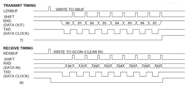
Figure 14.1. Serial Port Mode 0 Timing Diagram
