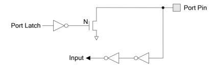
Figure 8.4. Open-Drain Mode Structure
