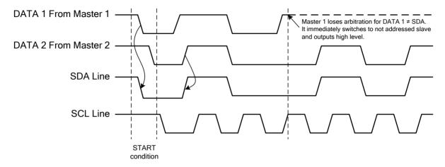
Figure 15.6. Arbitration Procedure of Two Masters
