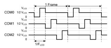
Figure 18.5. COM Driving Signals (1/3 Duty and 1/2 Bias)
