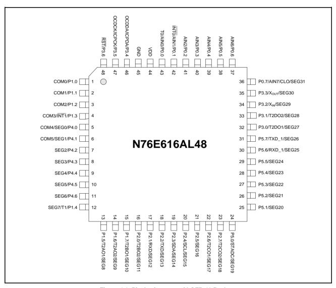
Figure 4.1. Pin Assignment of LQFP-48 Package
