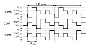
Figure 18.2. COM Driving Signals (1/3 Duty and 1/3 Bias)
