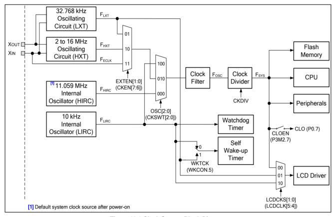
Figure 23.1 Clock System Block Diagram
