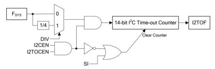
Figure 15.12. I<sup>2</sup>C Time-Out Counter
