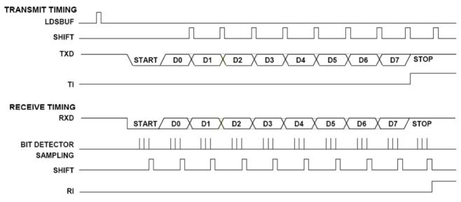
Figure 14.2. Serial Port Mode 1 Timing Diagram
