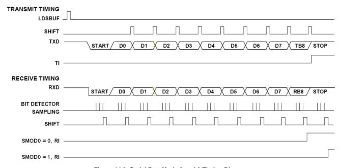
Figure 14.3. Serial Port Mode 2 and 3 Timing Diagram
