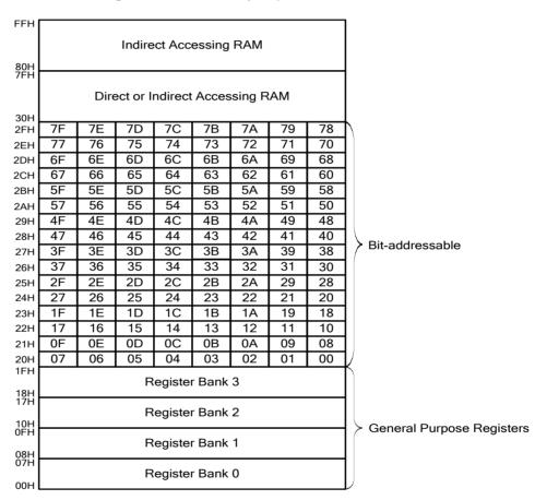
Figure 5.3. Internal 256 Bytes RAM Addressing
