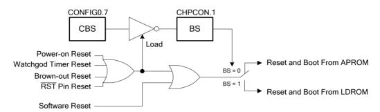
Figure 25.1. Boot Selecting Diagram
