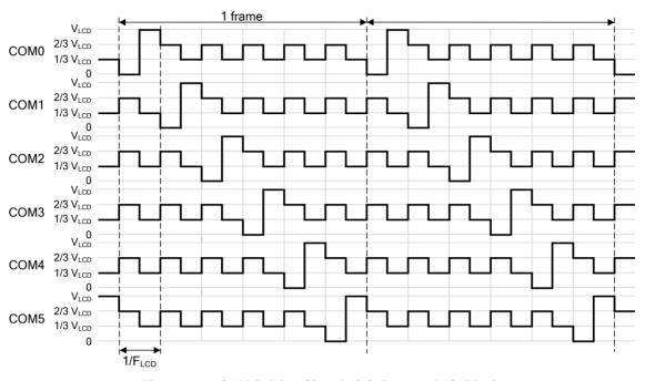
Figure 18.3. COM Driving Signals (1/6 Duty and 1/3 Bias)
