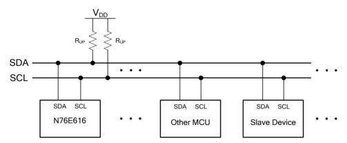
Figure 15.1. I<sup>2</sup>C Bus Interconnection
