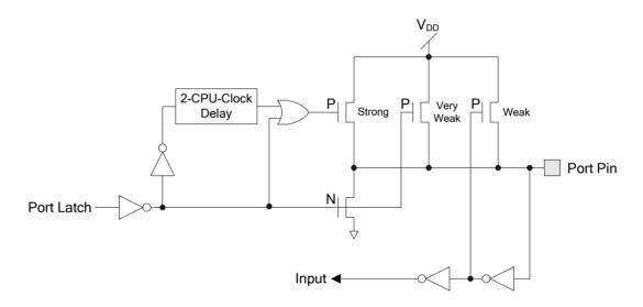
Figure 8.1. Quasi-Bidirectional Mode Structure
