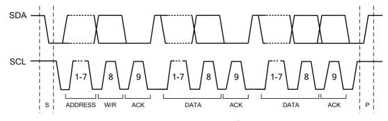
Figure 15.4. Data Format of One I<sup>2</sup>C Transfer
