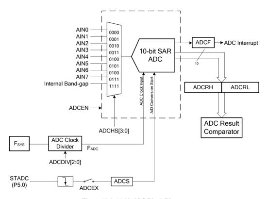
Figure 17.1. 10-bit ADC Block Diagram
