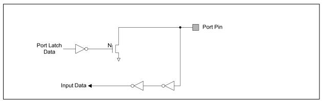
Figure 22-2: Open Drain Output
