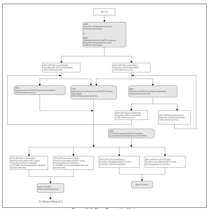
Figure 16-6: Slave Transmitter Mode
