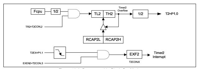
Figure 12-8: Programmable Clock-Out Mode
