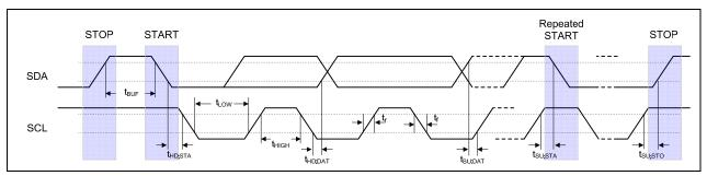
Figure 27-5: I2C Bus Timing
