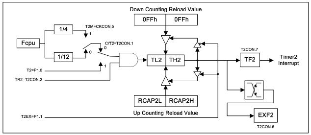
Figure 12-6: Timer 2 16-Bit Auto-reload Up/Down Counter
