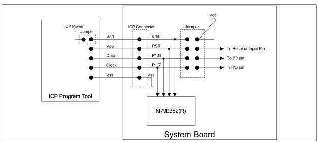
Figure 25-1: ICP Writer Tool connector pin assign
