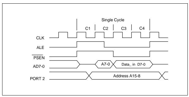
Figure 9-1: Single Cycle Instruction Timing
