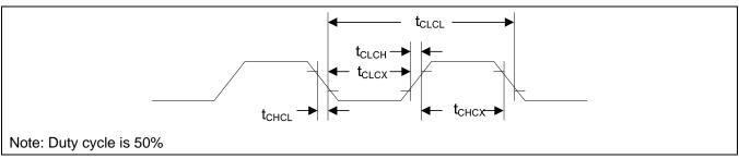
Figure 27-1 External clock characteristics
