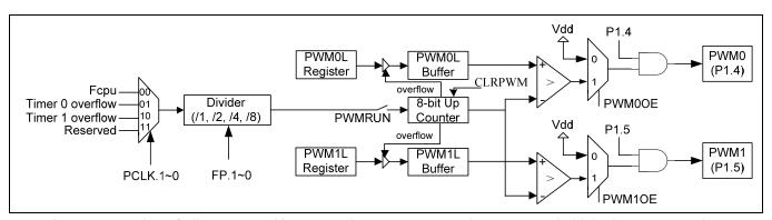
A compare value of all zeroes, 00H, causes the output to remain permanently high. A compare value of all ones, FFH, results in the PWM output remaining permanently low.
