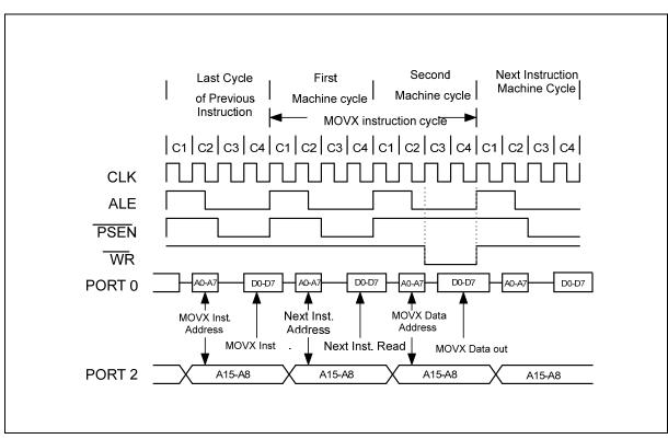
Figure 9-6: Data Memory Write with Stretch Value = 0
