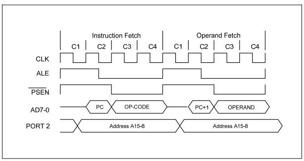
Figure 9-2: Two Cycle Instruction Timing
