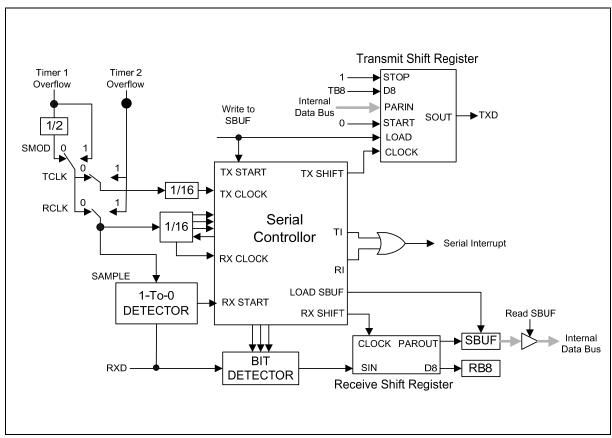
Figure 15-4: Uart Serial Port Mode 3
