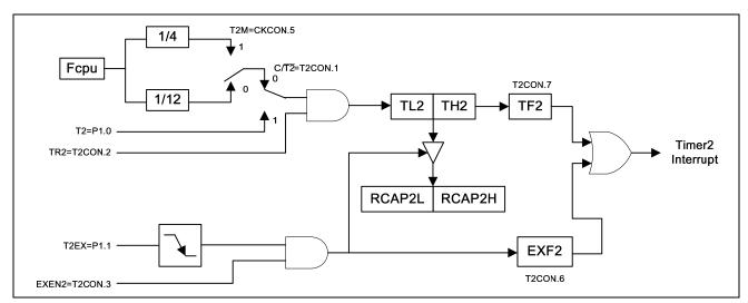
Figure 12-4: Timer 2 16-Bit Capture Mode
