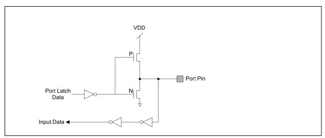
Figure 22-3: Push-Pull Output
