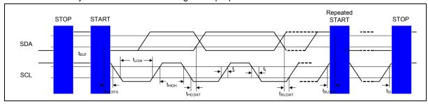
Figure 16-1: I2C Bus Timing
