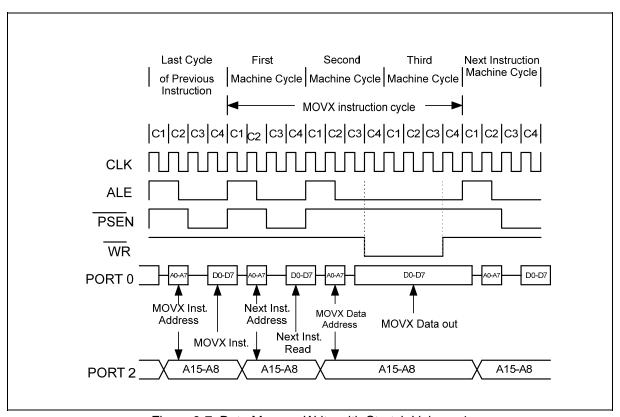
Figure 9-7: Data Memory Write with Stretch Value = 1
