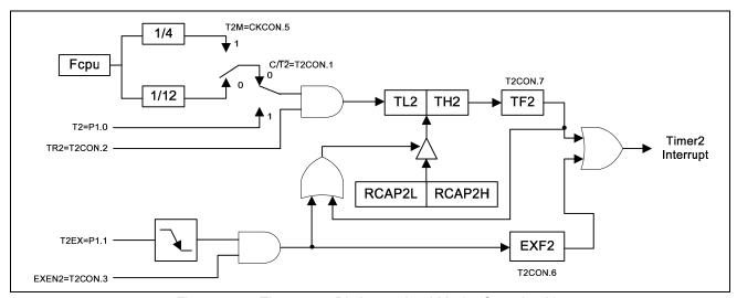
Figure 12-5: Timer 2 16-Bit Auto-reload Mode, Counting Up
