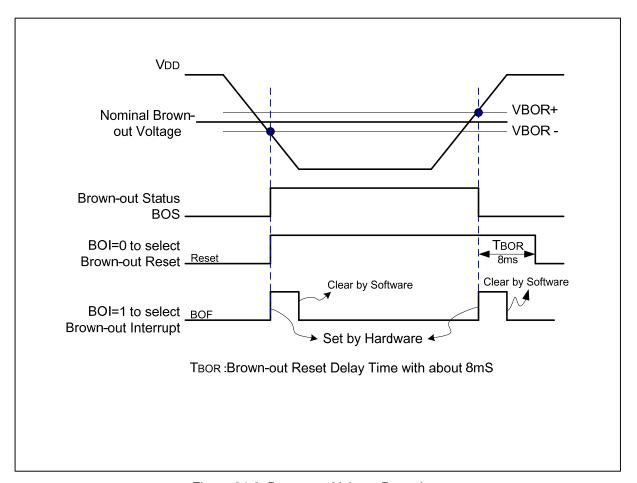
Figure 24-2: Brown-out Voltage Detection
