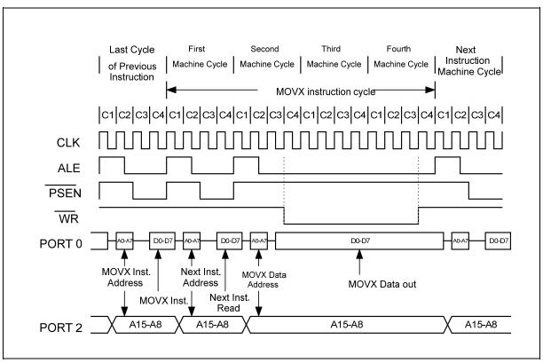
Figure 9-8: Data Memory Write with Stretch Value = 2
