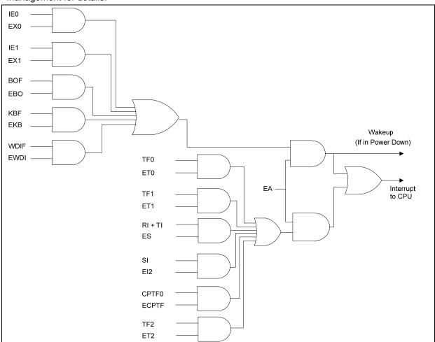
Figure 18- 1: Interrupt inputs
