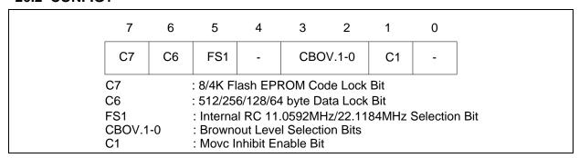
Figure 26-2: Config1 register bits
