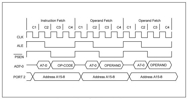
Figure 9-3: Three Cycle Instruction Timing
