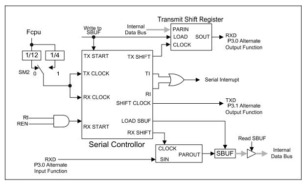
Figure 15-1: Uart Serial Port Mode 0
