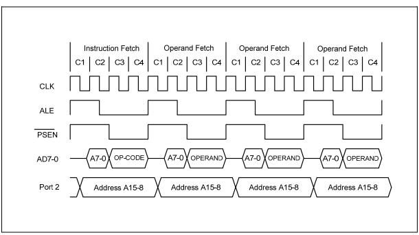
Figure 9-4: Four Cycle Instruction Timing
