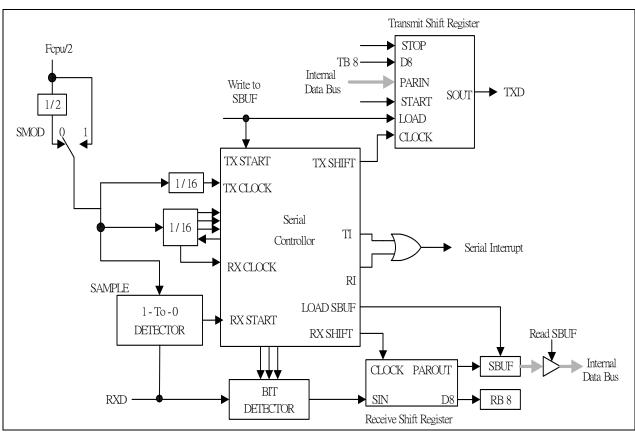
Figure 15-3: Uart Serial Port Mode 2
