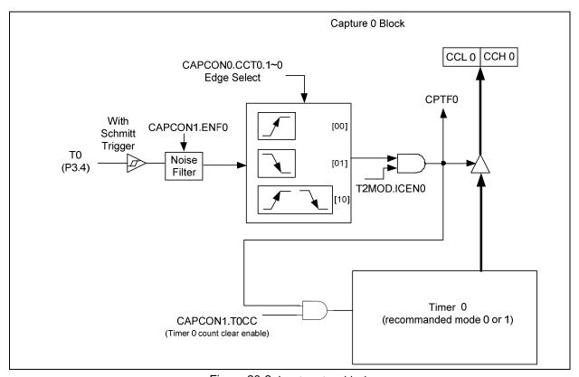
Figure 20-2: Input capture block
