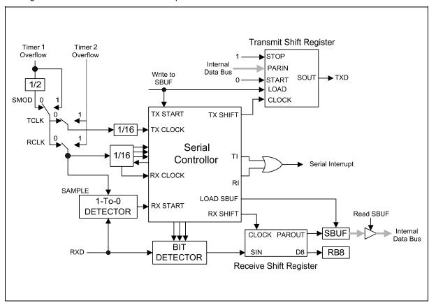
Figure 15-2: Uart Serial Port Mode 1
