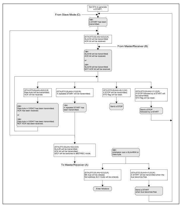
Figure 16-4: Master Transmitter Mode
