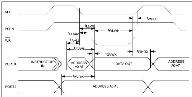
Figure 27-4 Data Memory Write Cycle
