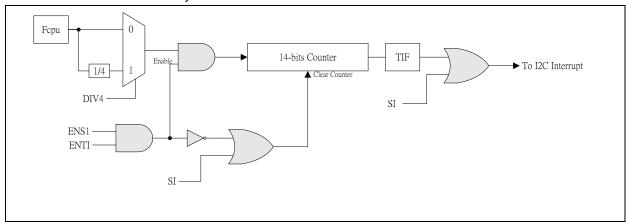
Figure 16-2: I2C Timer Count Block Diagram
