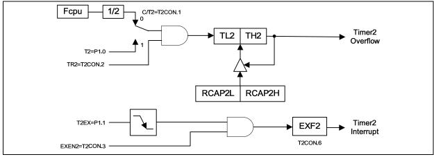
Figure 12-7: Baud Rate Generator Mode
