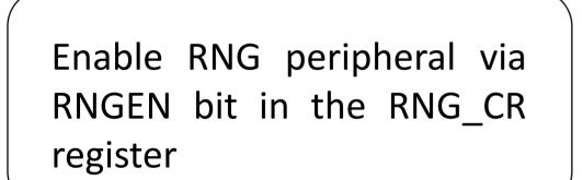
Note: The first random number generated after setting the RNGEN bit should not be used, according to FIPS (Federal Information Processing Standard Publication) PUB 140-2.
