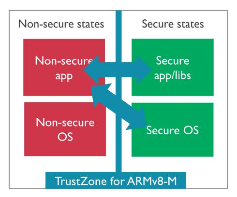
Secure transitions handled by the processor to maintain embedded class latency
